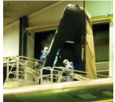
LM Aero staff painting the tail of a C-130J.
