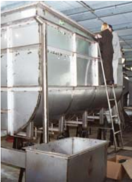
Judy Adler and Gary Brown inspect the new pea cooling equipment. Eliminating once-through cooling water for this equipment will save roughly 800,000 gallons of water per year.
